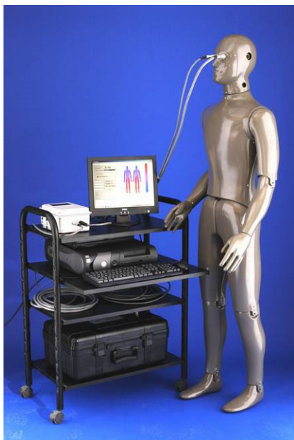
Figure 1, Thermal Manikin 'Newton'.
